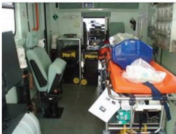
Fig. 4.2 A mobile intensive care trolley with equipment monitor, ventilator and infusion pumps which are fixed below the level of the patient. This provides a low centre of gravity and greater stability. The trolley fixes to the floor of the vehicle with a secure locking system and is not dependent on side-clamps or belt straps. (Picture courtesy of Reinout J. Mildner and Phil Wilson, Birmingham Children's Hospital NHS Foundation Trust.)
